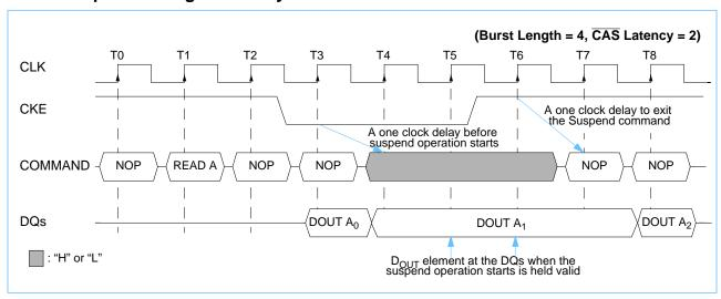
If Clock Suspend mode is initiated during a burst write operation, the input data is masked and is ignored until the Clock Suspend mode is exited.
