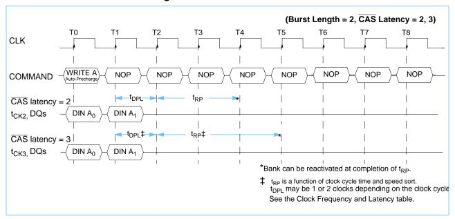
Similar to the Read Command, a Write Command with auto-precharge can not be interrupted by a command to the same bank. It can be interrupted by a Read or Write Command to a different bank, however. The precharge function will be initiated by the new command. After the Data-in to Active, delay, t<sub>DAL</sub>, is satisfied the bank may be reactivated.
